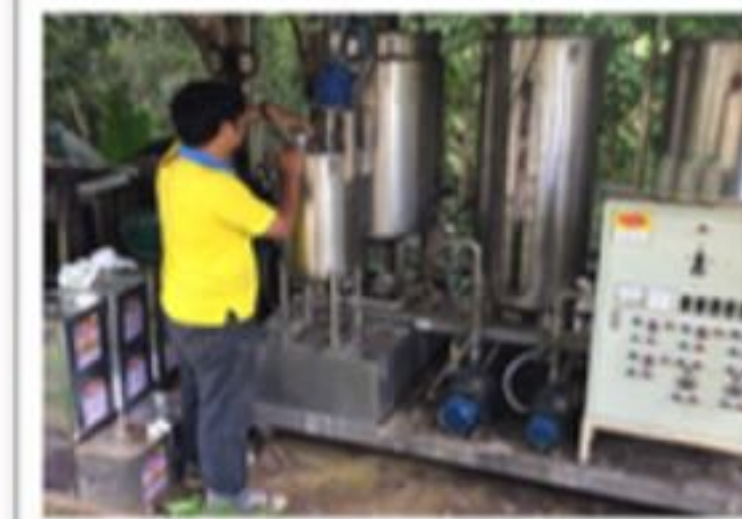
Biodiesel from waste cooking oil Reduce diesel 420 L/y GHG 1 tCO 2 /y 15,000 baht/y
