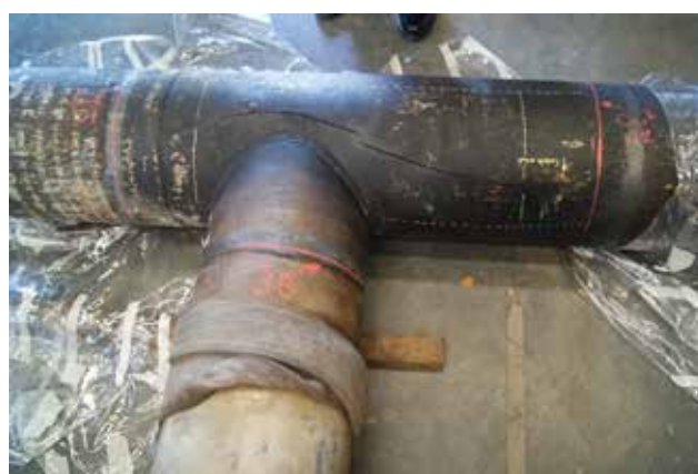
▲ Ruptured pipe sample for failure analysis
