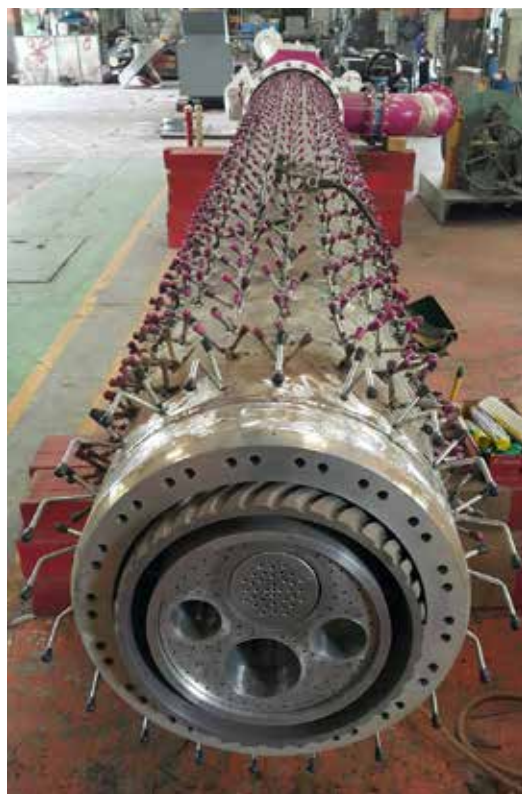
The kiln burner with anchors
