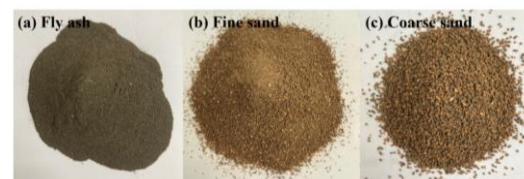
Figure 3 Photos of (a) FA, (b) fine sand and (c) coarse sand used in the production of paving blocks
