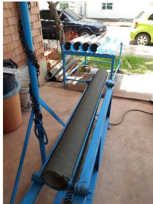
Figure 2 The green fiber cement pipe with 100 mm of inside diameter, 8 mm in thickness and 1200 mm in length
