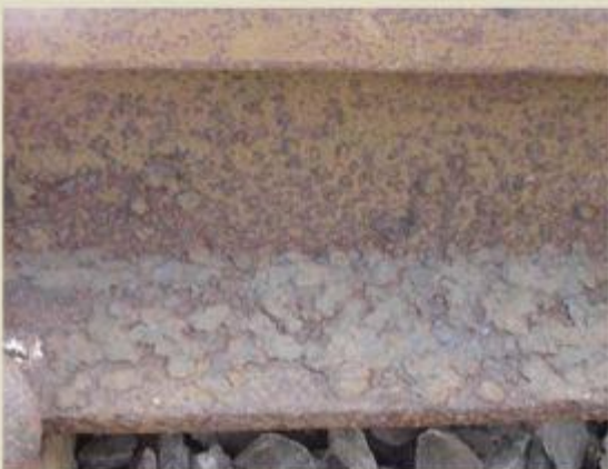
LESS SECTIONAL THINNING on weathering Cu-Mo rail.
