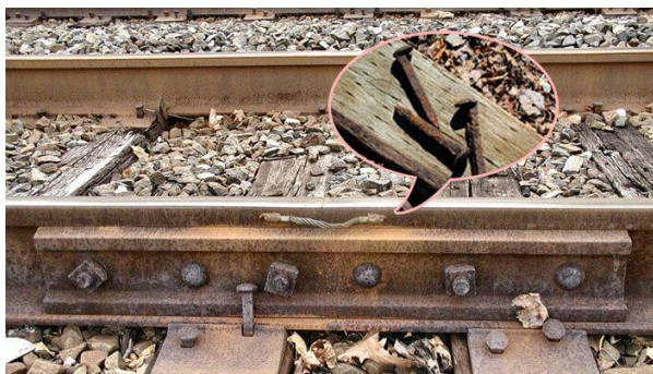
LESS SECTIONAL THINNING on weathering Cu-Mo rail.
