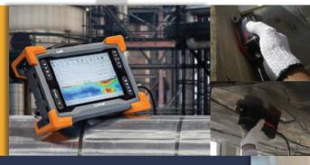
PULSED EDDY CURRENT No need to removeinsulation/fireproofing
