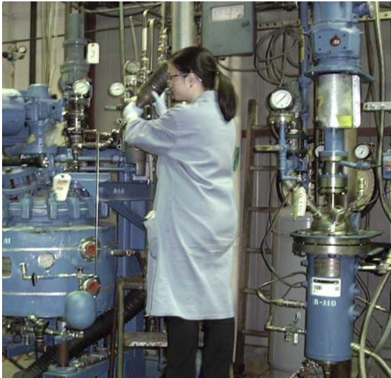
Engineer charging an additive to a reactor in a polybutadiene batch process
