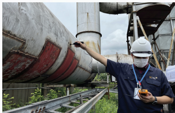
On-site gas collection trial
